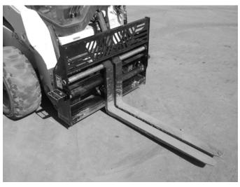
3. Activate the loader's auxiliary hydraulics to adjust the fork width to be wider or narrower in order to accommodate the load/object to be moved.
